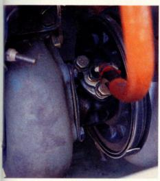
Chrome valve covers are part of the Millennium Edition package (top). The TIO-540's turbocharger has an automatic wastegate, so overboosting should not be a concern (above).
